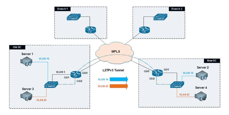
As demonstrated in the above diagram, the existing interface on VLAN 5, G0/1, continued to handle bidirectional traffic between branches and the old Data Center over MPLS. Similarly, the new interface G0/2 was configured as the source of Ethernet frames (VLANs) to be encapsulated into IP to tunnel that VLAN traffic over to the new data center.
