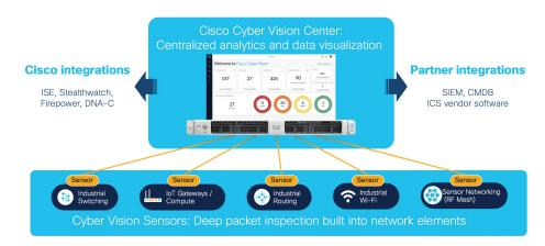
The benefits of Cisco Cyber Vision aren't limited to organizations with Cisco networks. The sensor can also be offered in a SPAN architecture with Cisco IC3000 hardware sensor appliance. This provides maximum deployment flexibility to meet your needs with your existing network, while giving you time to replace older switches with DPI-enabled network equipment that's capable of seeing everything that attaches to it.
